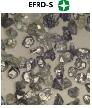
Our EFRD-S is a new generation diamond for use in resin bond and vitrified bond wheels. It has been produced to achieve micron grade cutting edges, a self-controlled micro fracturing and self-sharpening crystal, generating a free cutting action, and high bond retention. These special features result in a free cutting action at low temperatures , achieving a long life ,fast cutting and a premium surface finishclearly the product of choice EDA 2021
