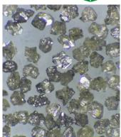
This resin bond has the highest friability within our range. Its characteristics promote microfracturing, making it very effective for high precision grinding applications whereby the surface finish is of high importance. When ordering with nickel, please order EDA 2020-30n, EDA 2020 - 56n. For copper EDA 2020-50c.
