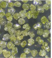
This green (jr1) diamond abrasive consists of crystals of irregular shape. Its rough and mosaic structure ensures excellent bond retention and its controlled micro-fracturing properties have made it the product of choice in most high quality resin and vitrified bonds for the wet & dry grinding of tungsten carbide. When ordering with nickel, order EDA 2023 - 30n, EDA 2023 - 56n. For copper EDA 2023-50c.
