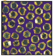
This is a specially synthesized highly well formed crystalline product almost entirely free of inclusions. It makes it an ideal crystal for applications requiring a high strength grit in sawing, drilling of the hardest stone, granite, refractories and reinforced concrete.
