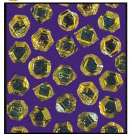
This is also a high strength product with a good thermal stability. A high percentage of perfectly formed cubo-octahedral crystals has established this product as the cost effective solution where performance is carefully measured. A free cutting, long lasting product.
