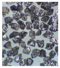
This is a strong blocky tetrahedral or octahedral crystal, with well developed faces and sharp cutting edges, for use in metal bonds and vitreous bonds, for the grinding, sharpening and honing of high-speed steels, superalloys, and cast irons over 45 HRC.
