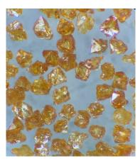
This is an amber colored crystal with a highly angular face rather than a blocky shape. This shape, combined with its high thermal stability and medium strength, makes it a highly versatile grit in wheel production using, vitrified, metal and electroplated single layer bonds.
